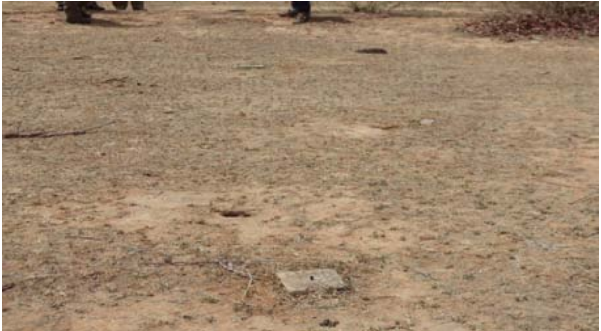
FIGURE 22 MEASURING SUBSIDENCE USING PILLARS, NAVEGAON RAJENDRA UNDERGROUND MINE
